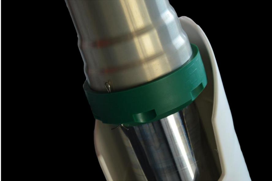
Check Mud scraper is positioned correctly and does not interfere with hole shot devices or other areas of the fork plastic shield.
